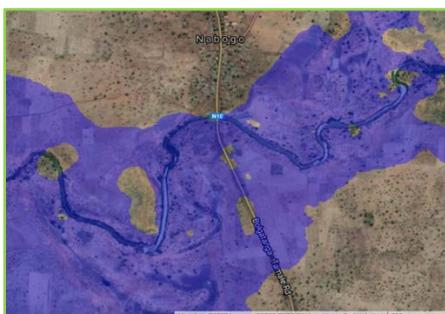
Example flood map layer for part of the Nabogo Basin in Northern region, Ghana. The image shows the area flooded (in blue) as a result of the Bagre Dam overflow in August – October 2018 as detected by satellite imagery
